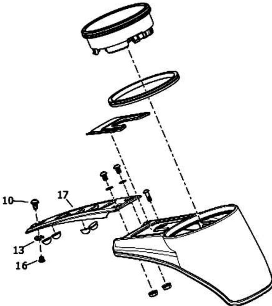
Loosen the rear screw (10) of the fuel tank dash cover (17).
